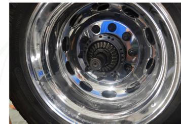
Remove axle shaft. Inspect wheel end, axle shaft and axle end for damage or excessive RTV and remove
